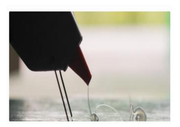
Acrylate-UV adhesives are resins which polymerize and therefore cure under UV light. These products are used mainly in industrial settings because they cure within seconds, allowing a high production output.
