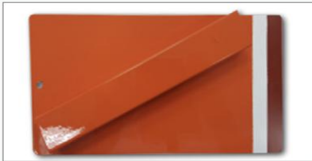
Figure 3: Orange high-gloss topcoat RR 3.3894-06 on steel
